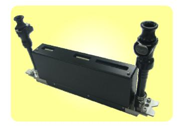
KJ4A-TA06ATB-STDC inkjet printhead is designed for high speed single-pass and multi-pass applications with UV based ink. It delivers 600 dpi x 600 dpi resolution at 50 m/min by making use of 2,656 nozzles arranged across 108 mm width.
